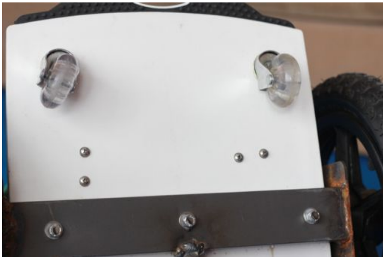
Close up of the underside. Front casters are seen at the top. Metal frame, which wheels are mounted to is below. The four small screws are where the BUMBO is attached to the cutting board.
