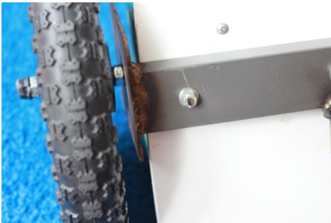
Close up of the main wheels. They attach to the metal plate, which is welded to the metal bar on the underside of the cutting board base.
