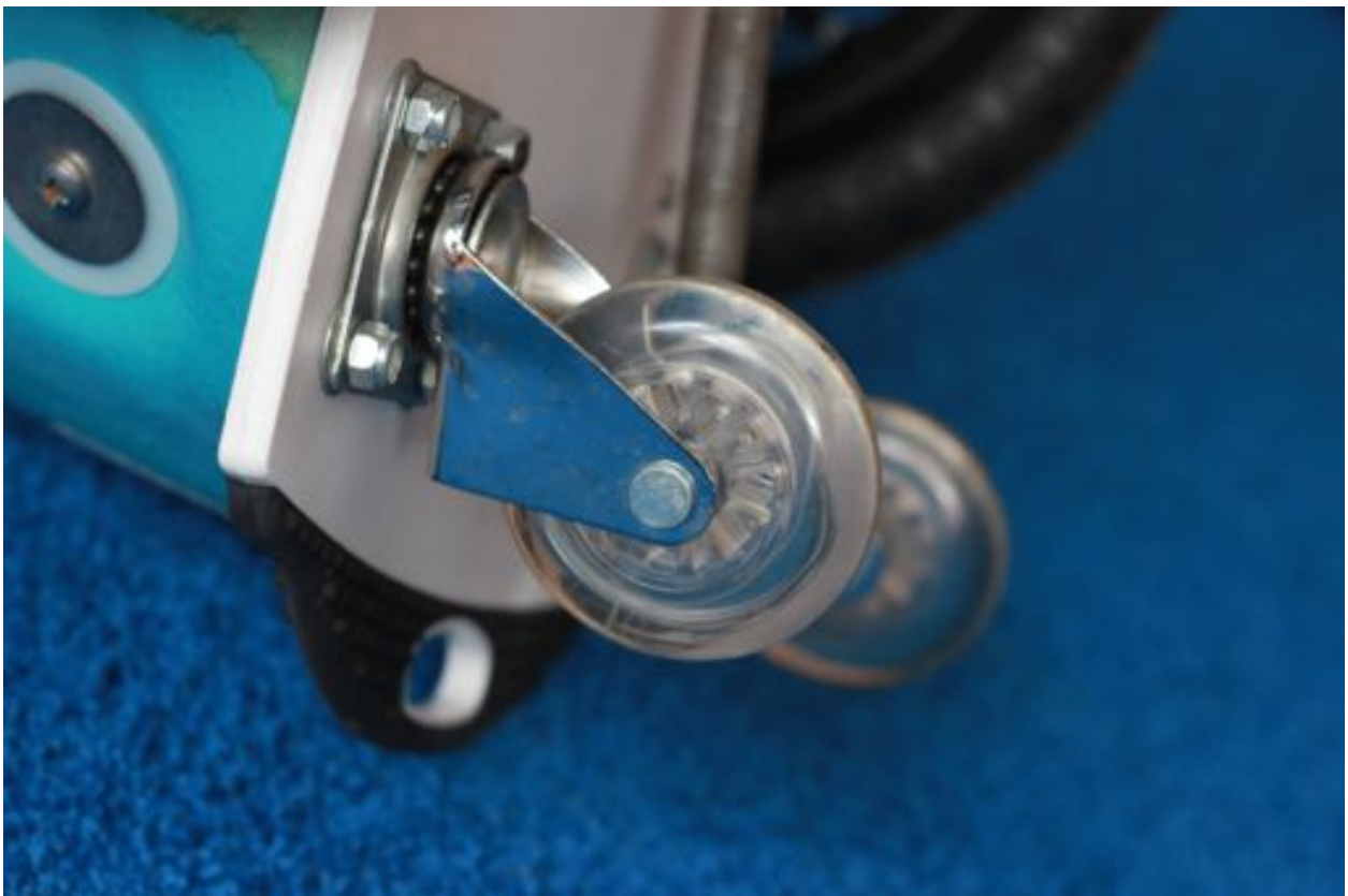
Close up of the larger back casters (these sit on the floor at all times)
