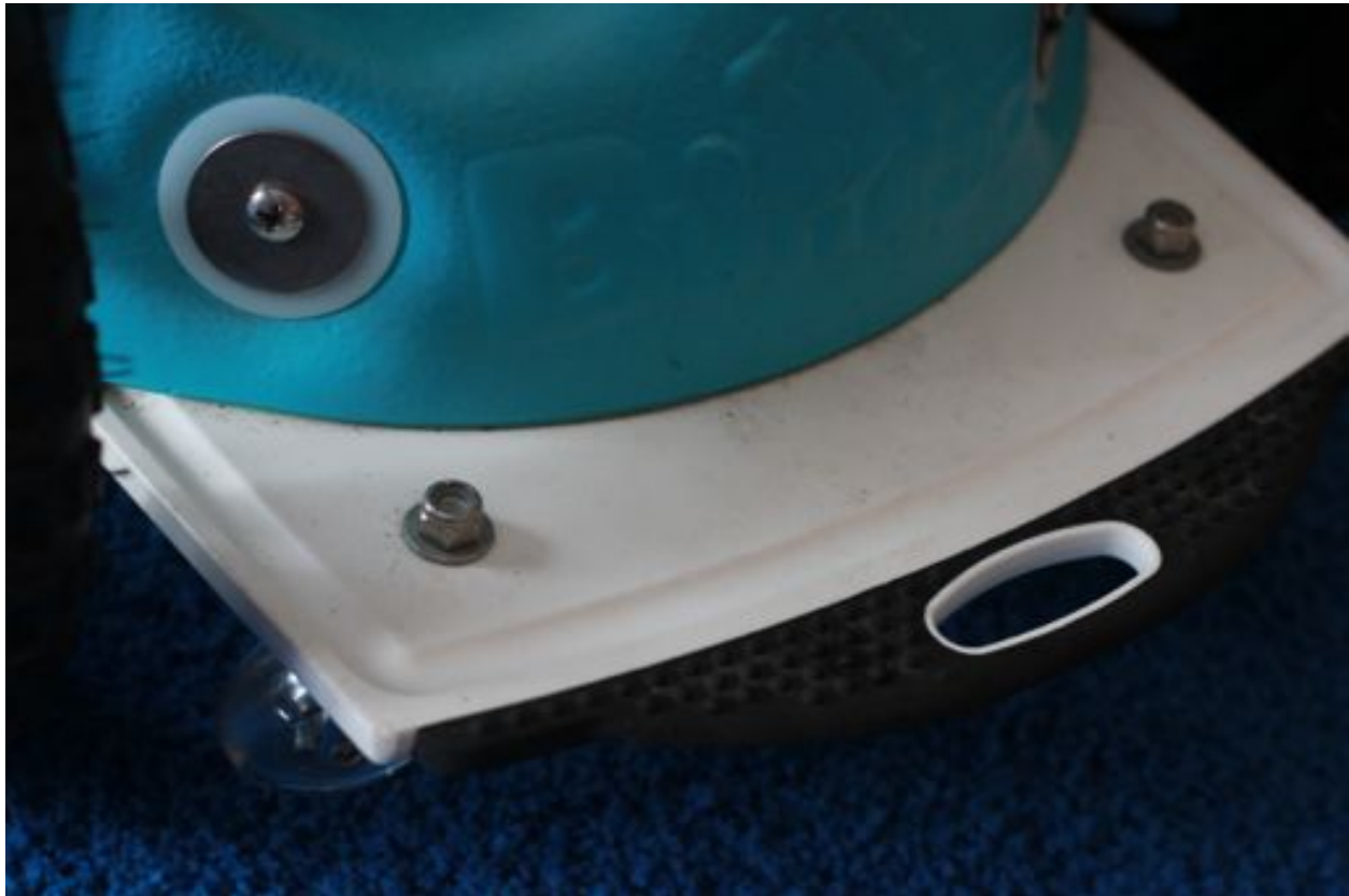
The base is a sturdy plastic cutting board. The large screws are holding the front casters in place. The screws on the circular metal piece (on the BUMBO itself) are holding the BOMBO to the board.
